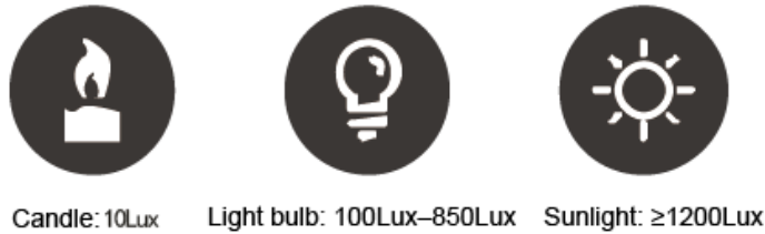
Figure 2-4 Ambient illumination requirement
